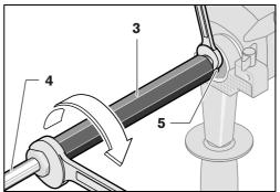
Screw the stirrer paddle 4 with the adapter 3 onto the drive spindle 5. Hold the drive spindle 5 in place with an open-end spanner (size 17 mm) and tighten the adapter 3 and the stirrer paddle 4 with a second openend spanner (size 24 mm).
